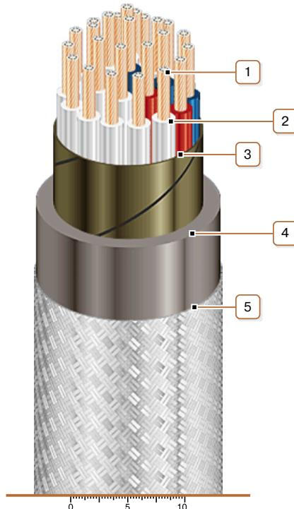
1. Copper multiwire conductor
