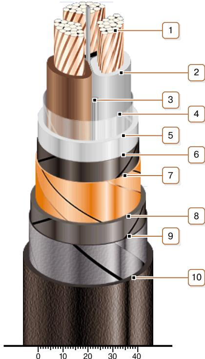
1. Copper multiwire compact conductor
