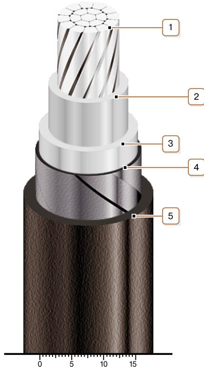
1. Aluminium multiwire compacted conductor
