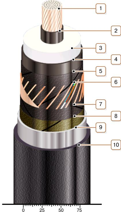
**1. Copper multiwire compact conductor**
