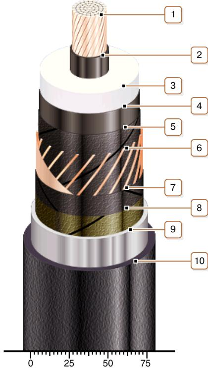
**1. Copper multiwire compact conductor**
