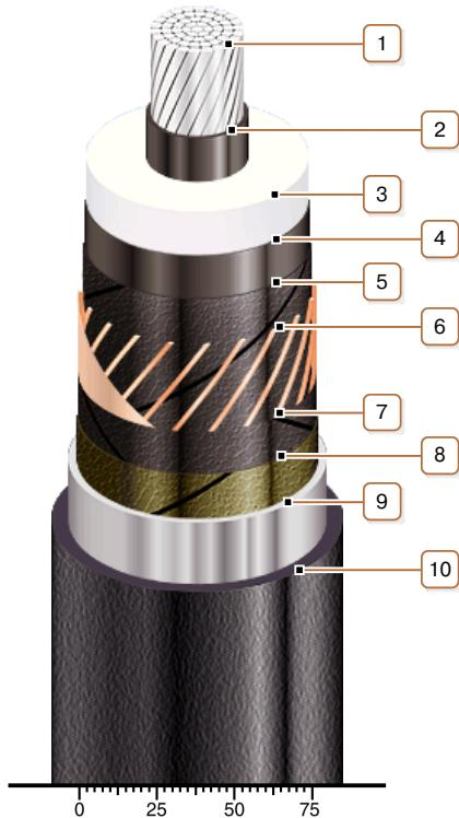
**1. Aluminium multiwire compacted conductor**
