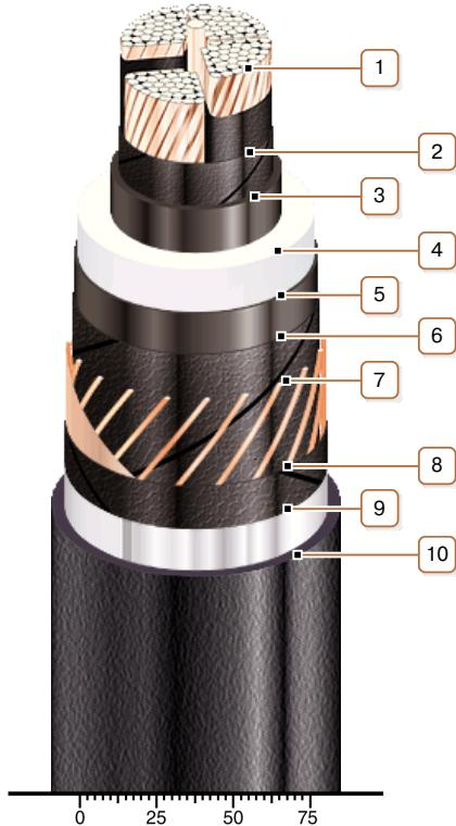
**1. Copper segmentary multiwire compact conductor**
