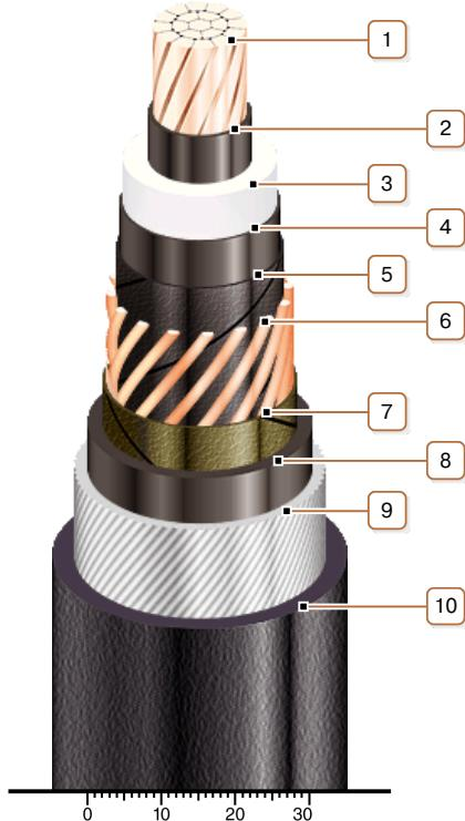
**1. Copper multiwire compact conductor**
