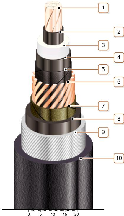
**1. Copper multiwire compact conductor**
