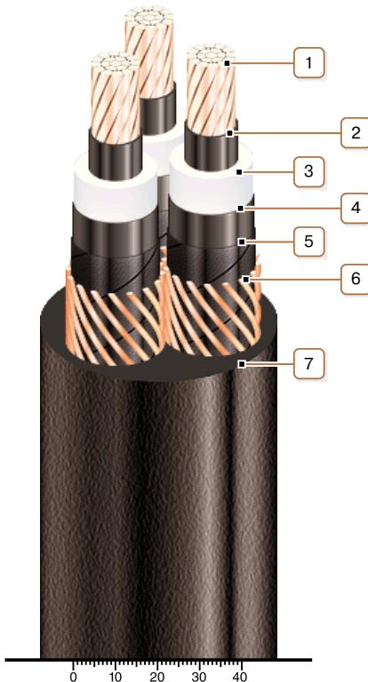
**CONSTRUCTION****1. Copper multiwire compact conductor***Note: It is possible to manufacture cable with sealed conductors.***2. Inner extruded semiconducting layer****3. XLPE insulation****4. Outer extruded semiconducting layer****5. Lapping layer of semiconductive swellable tape****6. Copper screen****7. PVC compound outer sheath***Note: Conductor twisting is not illustrated*
