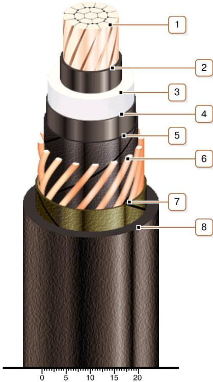
**CONSTRUCTION****1. Copper multiwire compact conductor***Note: It is possible to manufacture cable with sealed conductor.***2. Inner extruded semiconducting layer****3. XLPE insulation****4. Outer extruded semiconducting layer****5. Lapping layer of semiconductive swellable tape****6. Copper screen****7. Lapping layer of nonwoven cloth tape****8. PVC compound outer sheath**
