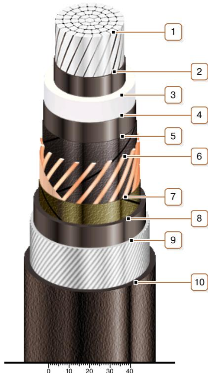
1. **Aluminium multiwire compacted conductor**
