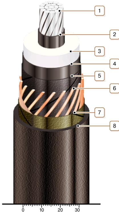
**CONSTRUCTION****1. Aluminium multiwire compacted conductor***Notes:*
