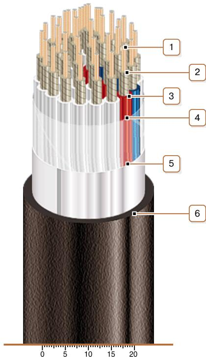
1. Copper multiwire conductor
