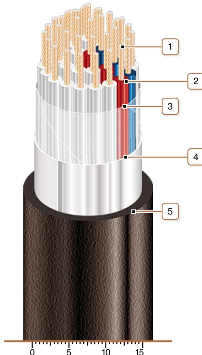
1. Copper multiwire conductor
