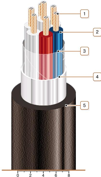
1. Copper multiwire conductor
