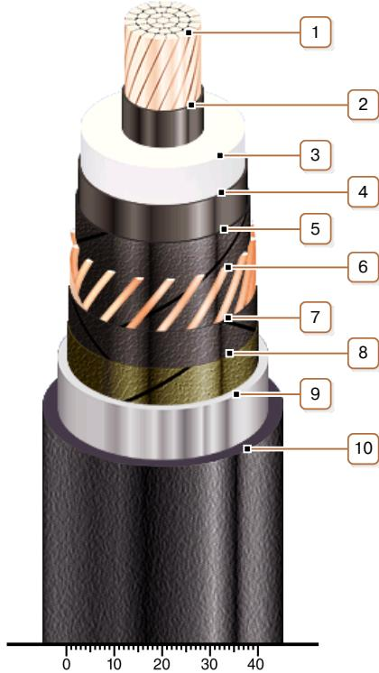
**1. Copper multiwire compact conductor**
