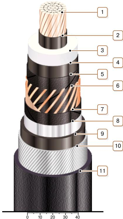
**1. Copper multiwire compact conductor**
