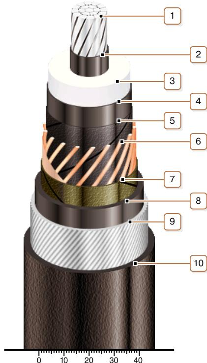
**1. Aluminium multiwire compacted conductor**
