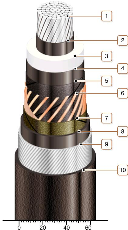
1. **Aluminium multiwire compacted conductor**
